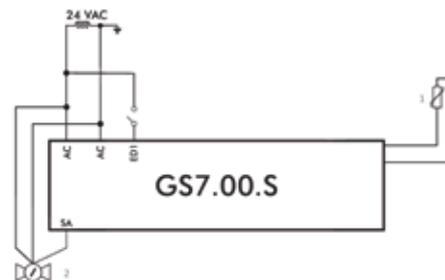
**FAN-COIL CONTROL AND VAV BOX ACTIVATION**
